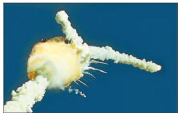
**What happened:** A booster rocket seal failed and burning fuel breached the external tank, which disintegrated, as did the shuttle. The crew cabin slammed into the ocean from about 12 miles up.
